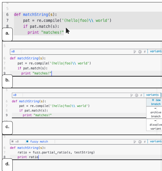
Figure 5. Creating a variant box in Variolite. In (a) the user selects a section of code and selects the command “wrap in variant”. In (b) this places a box around the code, which can be used to keep multiple versions of that chunk of code (c, d).
