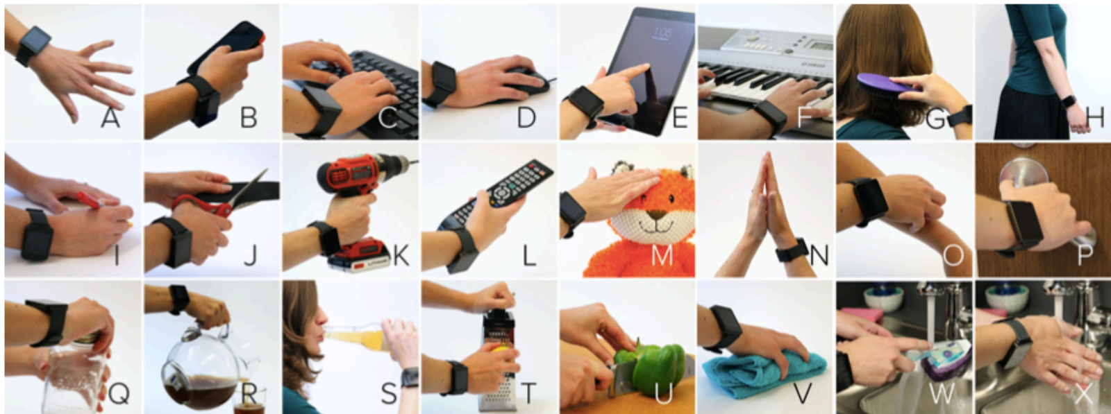
Figure 1. In this work, we investigate the feasibility of sensing 25 hand activities using commodity smartwatches, which are uniquely positioned to capture such fine-grained activity. Activity names are provided in Figure 3. The 25th hand activity we evaluated, brushing teeth (Y), is not shown here.
