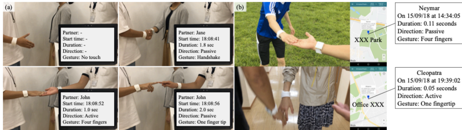
Figure 1: EnhancedTouchX: (a) Identifying a partner, a direction (from one initiating the touch (active touch) to the one being touched (passive touch)), and gestures of interpersonal touch of the left user; (b) Interpersonal touch logging system using a smartphone (EnhancedTouchLog).
