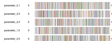
Figure 7: Shows horizontally the sampling range and in grey vertical lines all the values that occurred in sampling the parameter range. The coloured vertical lines represent values achieved in the clusters. A selected cluster gets a colour assigned and parameter values that were used for models assigned to that cluster get coloured accordingly. As you can see here, it is very hard to detect, which lines have which colour and therefore are related to which cluster. Additionally because of the colour soup, it is hard to see any patterns for the different coloured bars.
