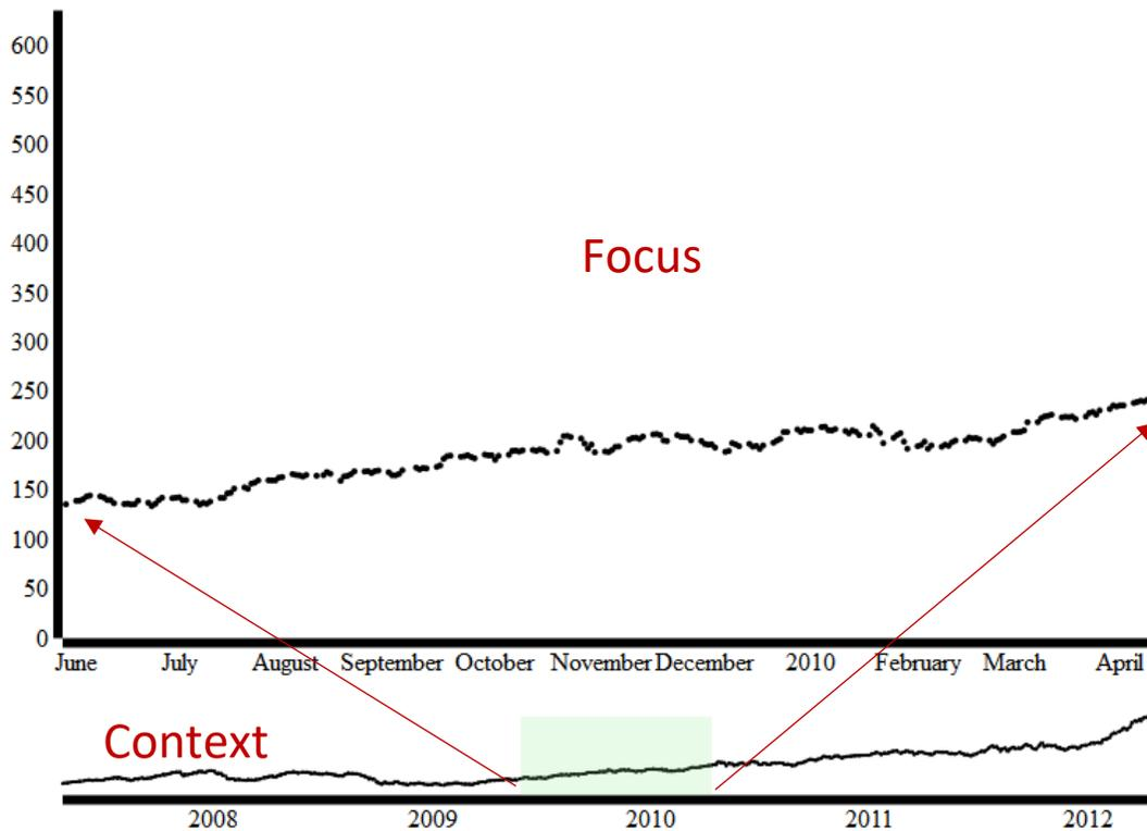
Brushing is conveniently implemented in D3 via the *brush* component. This creates an element that works similar to an axis and allows the user to select subsets of the data with their mouse.
