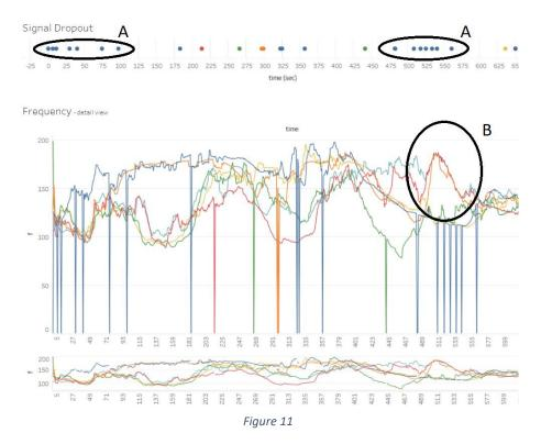
At the first glance, the technician notices, that the blue dancer has significantly more signal dropouts, than the other dancers. Moreover, the dropouts are suspiciously located at the very beginning, and near the end of the performance (annotation A). Dropouts of the other dancers are not so critical.
