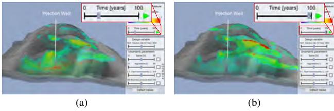
Fig. 2. Visualization of different time steps of the simulation result. Time steps can be manually selected with a slider (close-up) or automatically displayed as an animation sequence. CO<sub>2</sub> saturation is shown.
