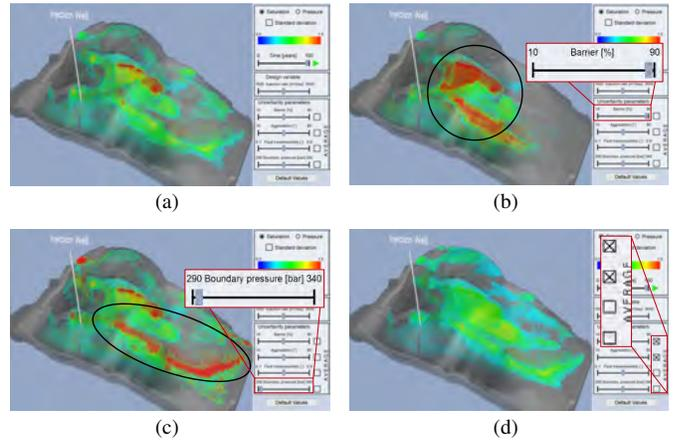
Fig. 3. Exploring the parameter space. (a) The CO<sub>2</sub> saturation at the end of the time range with default parameters. Parameters of the simulation like (b) the percentage of barriers or (c) the boundary pressure can be interactively changed and their influence observed, e.g., areas with increased CO<sub>2</sub> saturation (marked black). (d) It is also possible to average parameters instead of setting them to specific values.
