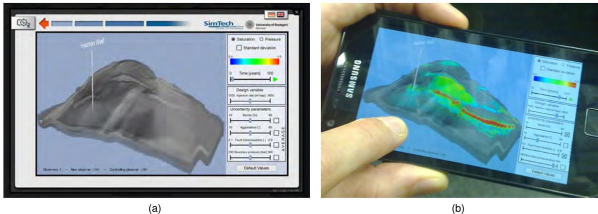
Fig. 1. The developed software allows the user to interactively change uncertain parameters of the simulation. The resulting CO<sub>2</sub> concentration in the storage site is visualized in combination with the geological context of the storage site. The tool supports remote access. It is possible to interact with it via (a) web browser or (b) mobile device, which makes it easy to provide the public with access to the simulation. This may help communicate risks of the simulated technology.
